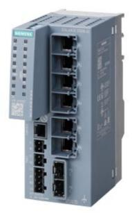
SCALANCE SC636-2C Industrial Security Appliance; For protection of devices and networks in discrete manufacturing and the process industry For protection of industrial communication with firewall; Further functions: Address translation (NAT/NAPT); Connection to SINEMA RC; 4x ports electrical 10/100/1000 Mbps RJ45 and 2x combo port electrical or optical; 10/100/1000 Mbps RJ45 or 100 Mbps SFP or 1000 Mbps SFP
