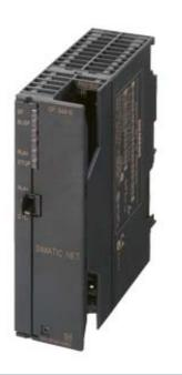
COMMUNICATIONSPROCESSOR CP343-5 FOR CONNECTING SIMATIC S7-300 TO PROFIBUS, FMS, S5-COMPATIBLE PG/OP AND S7 COMMUNICATION 12 MBAUD, SINGLE-WIDTH
