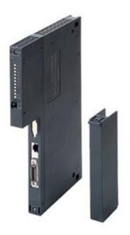
COMMUNICATIONSPROCESSOR CP443-1 FOR CONNECTION OF SIMATIC S7-400 W. IND. ETHERN.,ISO/TCP/IP AND UDP S7 COMM.,FETCH/WRITE, DIAGNOST. EXPANSIONS, SEND/RECEIVE, WITH AND W/O RFC 1006, MULTICAST, NTP, INITIALIZING THROUGH LAN ACCESS PROTECTION USING IP-ACCESS LIST, 10/100 MBIT
