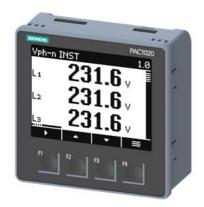
SENTRON PAC1020 96X96 mm Power Monitoring Device Panel mount type for measurement of electr. values Protocol: Modbus RTU With graphical display Un max: 400/230V 45-65Hz Input current 5A AC Power Supply 85V - 276V AC Terminal blocks
