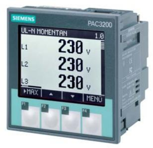
SENTRON, measuring device, 7KM PAC3200, LCD, L-L: 500 V, L-N: 289 V, 5 A, 3-phase, Modbus TCP, optional Modbus RTU / PROFINET / PROFIBUS, apparent/ active/reactive energy, class 0.5 acc. to IEC61557-12 or class 0.5s acc. to IEC62053-22, ext-low volt. pwr sup. unit DC, screw terminals
