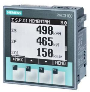
SENTRON, measuring device, 7KM PAC3100, LCD, L-L: 480 V, L-N: 277 V, 3-phase, Modbus RTU, active/reactive energy, class 1 acc. to IEC 61557-12 & 62053- 21, wide-range power sup. unit AC/DC, screw terminals
