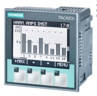
SENTRON, measuring device, 7KM PAC4200, LCD, L-L: 690 V, L-N: 400 V, 5 A, 3-phase, Modbus TCP, optional Modbus RTU / PROFINET / PROFIBUS / DI/DO, apparent/active/reactive energy / cos phi, harmonics: 3.-31., THD, class 0.2 acc. to IEC61557-12 or cl. 0.2S acc. to IEC62053-22, wide-range pwr sup. unit AC/DC, screw terminals
