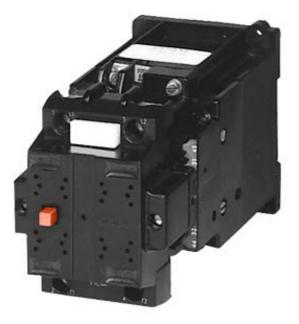
CONTACTOR, SIZE 2, 2-POLE DC-3 AND 5, 32A AUXILIARY SWITCH 22 (2NO+2NC) DC OPERATION DC 24V WORKING RANGE 0.85 - 1.1 UN
