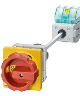
EMERG. STOP SWITCH 3-POLE IU=63, P/AC-23A AT 400V=22KW FLOOR MOUNTING DIN RAIL/TWO-HOLE MOUNTING ROTARY ACTUATOR RED/YELLOW (EMERG. STOP)
