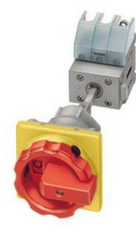
MAIN/EMERG. STOP SWITCH 3-POLE IU=100, P/AC-23A AT 400V=37KW FLOOR MOUNTING DIN RAIL/TWO-HOLE MOUNTING ROTARY ACTUATOR RED/YELLOW (EMERG. STOP)
