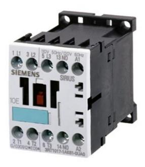
CONTACT. 3-PH., 4KW/400V, 1NC, 120 V AC 50/60 HZ, 3-POLE, SIZE S00, SCREW CONNECTION
