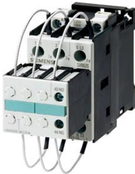
CAPACITOR SW. CONTACTOR, AC-6, 25KVAR/400V, 24V, 50HZ, 3-POLE, SIZE S0
