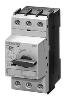
CIRCUIT-BREAKER SIZE S0, FOR MOTOR PROTECTION, CLASS 10, A-REL. 2.8...4A, N-REL. 52A, SCREW TERMINAL, STANDARD SWITCHING CAPACITY
