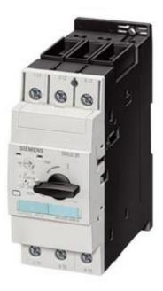
CIRCUIT-BREAKER, SIZE S2, FOR MOTOR PROTECTION, CLASS 20, A-RELEASE 14...20 A, N-RELEASE 260 A, SCREW CONNECTION, STANDARD BEAKING CAPACITY
