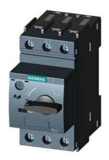
CIRCUIT-BREAKER SZ S00, FOR MOTOR PROTECTION, CLASS 10, A-REL. 0.18...0.25A, N-RELEASE3.3A SCREW CONNECTION, STANDARD SW. CAPACITY
