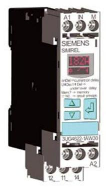
Digital monitoring relay Current monitoring, 22.5 mm from 0.05-10 A AC/DC 0vershoot and undershoot 24 to 240 V AC/DC 50 to 60 Hz DC and AC ON delay and noise pulses delay 0.1 to 20 s Hysteresis 0.01 to 5 A 1 change-over contact with or without fault buffer screw terminal Successor product for 3UG3522-1AL20, 3UG3522-1AG20 and 3UG3522-1AC48-0AA1
