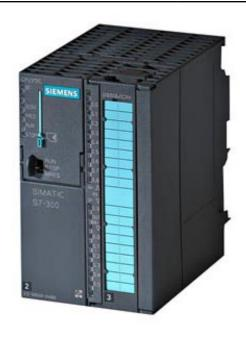
SIMATIC S7-300, CPU 312C COMPACT CPU WITH MPI, 10 DI/6 DO, 2 FAST COUNTERS (10 KHZ), INTEGRATED 24V DC POWER SUPPLY, 32 KBYTE WORKING MEMORY, FRONT CONNECTOR (1 X 40PIN) AND MICRO MEMORY CARD REQUIRED
