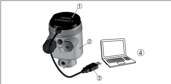
Fig. 45: Connection of the PC via VEGACONNECT and USB
