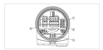
Electronics and connection compartment, single chamber housing
