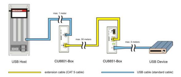
This configuration (1) contains no additional USB hub. The maximal distance of extension is 56 meters: 1 meter of cable to the extension box CU8801; up to 50 meters extension cable and 5 meters from extension box CU8851 to USB device.
