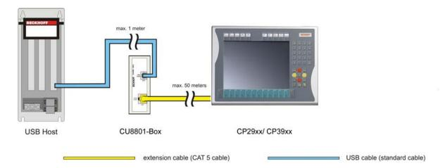
This configuration shows a CP29xx/ CP39xx Control Panel connected to the CU8801 extension box. The maximal distance of extension is 51 meters: 1 meter of cable from the host computer to the CU8801 extension box; up to 50 meters extension cable to the Control Panel.
