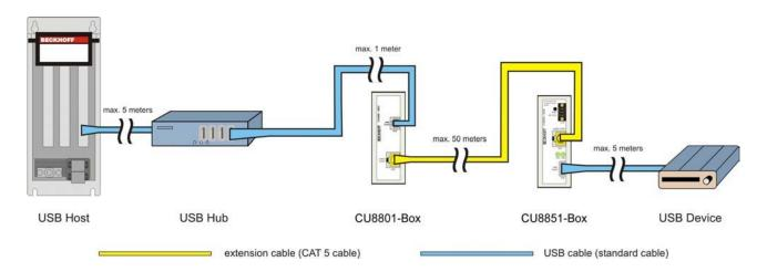
This configuration (2) contains an additional USB hub. The USB hub is connected directly to the host computer. The maximal distance of extension is 61 meters: 5 meters of cable from USB host to the USB hub; 1 meter cable to the extension box CU8801; up to 50 meters extension cable and 5 meters from extension box CU8851 to USB device.
