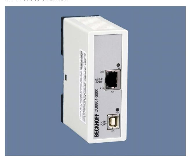
The Beckhoff CU8801-0000 USB2.0-Extender-Tx allows to extend the limits of USB cable length. Standard USB cable are specified for cable length up to 5 meters. For some industrial applications there is need for longer distances. This box can extend the distance up to 50 meters. This box sends the USB signals from input port to the receiver unit. Other outstanding features are:
