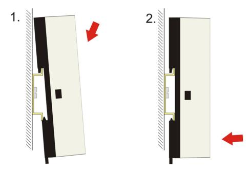
To release the CU8801-0000 from the mounting rail:
