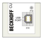
The USB2.0-Extender-Tx does not need any additional power supply. The power supply (5 V DC) is realized by the USB connector. The LED **P10** lights green when power supply is connected.
