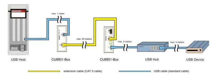
The third configuration (3) has nearly the same structure than configuration 2. The USB hub is connected after the extension. The maximal distance is also 61 meters: 1 meter of cable from USB host to the USB extension box CU8801; up to 50 meters extension cable; 5 meters from extension box CU8851 to USB hub and 5 meters of cable to the USB device.
