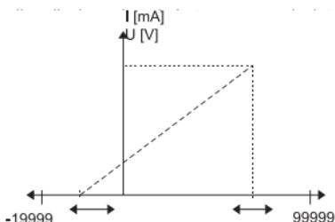
Displayed value can be freely adjusted to the input value inside the display range.
