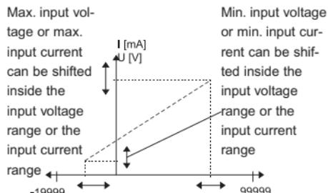
Displayed value can be freely adjusted to the input value inside the display range.
