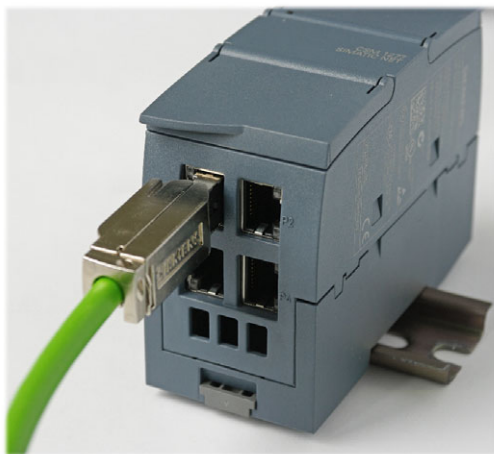
Figura 4-7 Enchufar el IE FC RJ45 Plug 180
